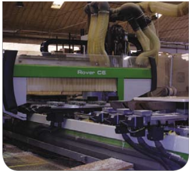
Silwood's investment in automated material handling and a Rover C machining center have allowed the company to offset high labor costs and expand market opportunities.
