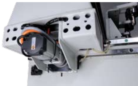
X Axis helical rack & pinion with precision linear guides and digital servo motors guarantee high precision and high quality cut
