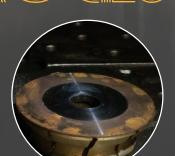
Diamut tooling is highly designed to achieve tolerances that are extremely tight. The tool redressing process requires extremely skilled operators using a sequence of precision, custom-engineered machines to match original tool profiles precisely.
